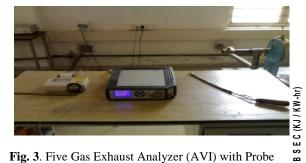
Fig. 3. Five Gas Exhaust Analyzer (AVI) with Probe
